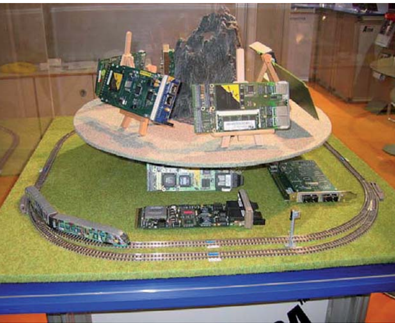
This railway-demonstration showed how easy, flexible and scalable a control application can be implemented with a standard MicroTCA system
